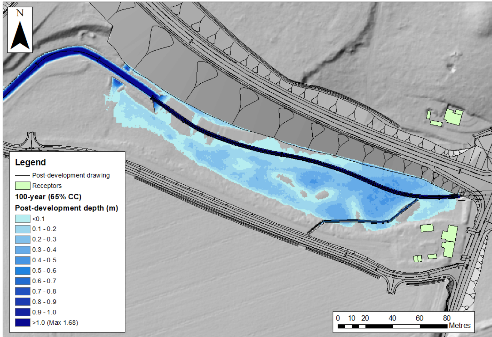
Figure A.6 Maximum predicted depths between A11 and Cantley Lane South for post-development scenario
