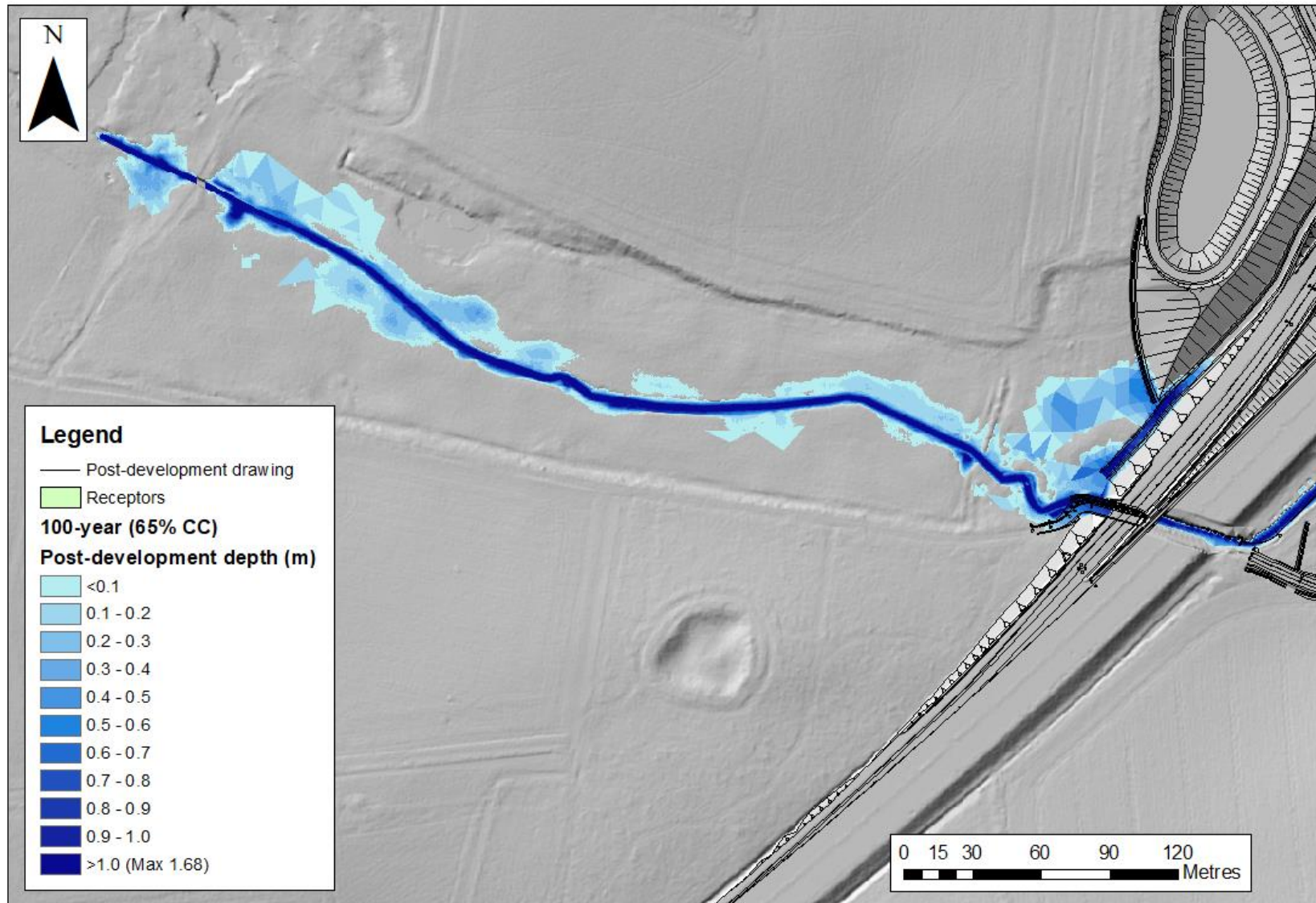
Figure A.4 Maximum predicted depths between upstream boundary and A11 for post-development scenario
