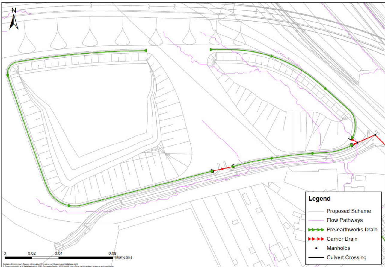
Figure 8-10: Proposed earth bund drainage arrangements
